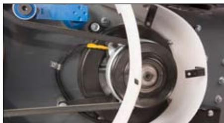
Fully controllable clutch - eliminates problems with marking the floor on start-up
