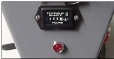
0-9999 hour meter easily monitors both Operator and machine times.
